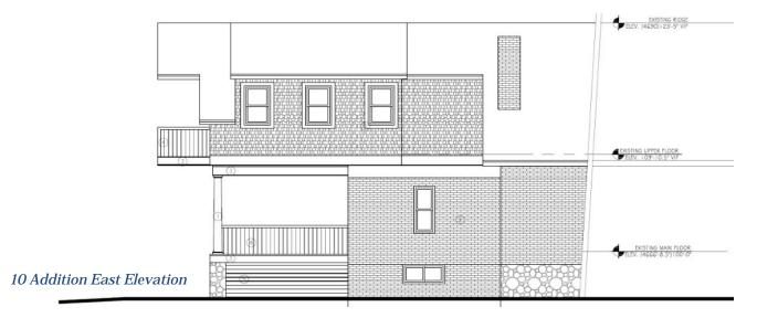
Most of the addition would be clad in wood shingles similar to those in the gables of the historic building, though these would have a consistent square edge instead of the fish scale shape seen on the historic gables.
