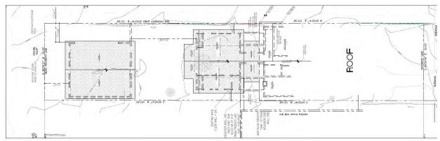
7: Site Plan with new construction shown in shaded areas
